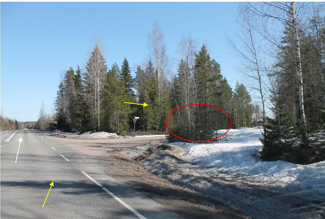
Pos 20/Pic 58. Turning from road 23 toward Rautalammentie. https://goo.gl/maps/vY6EfRHcbuutHDga8 Bridge detour. Marked trees need to cut. During the wintertime road need extra maintenance. Yellow arrow points driving direction for towers. White arrow points driving direction for blades.
