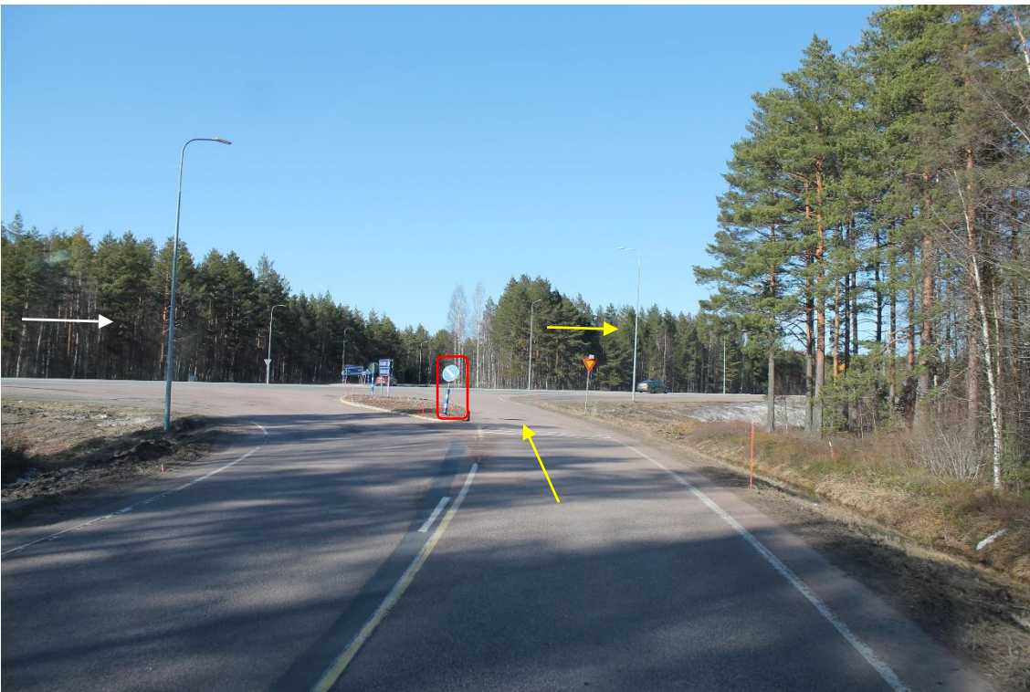
Pos 19/Pic 56. Turning from road 261 toward road 23. https://goo.gl/maps/69GubpAtixrrSAQy6 Bridge detour. Marked sign need to be removed. Yellow arrow points driving direction for towers. White arrow points driving direction for blades.
