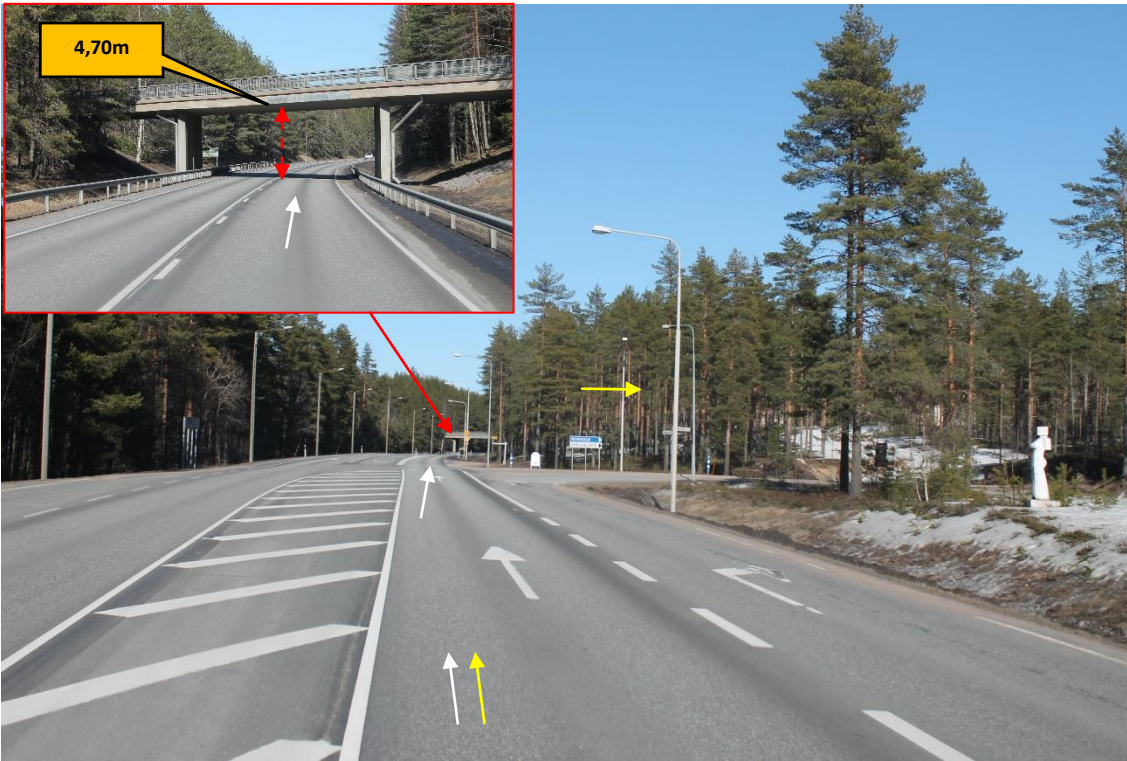
Pos 15/Pic 49. Turning from road 23 toward Varuskunnantie. https://goo.gl/maps/FQHZRCLFP4kQ6ogL7 Bridge detour. White arrow points driving direction for blades. Yellow arrow points driving direction for towers.
