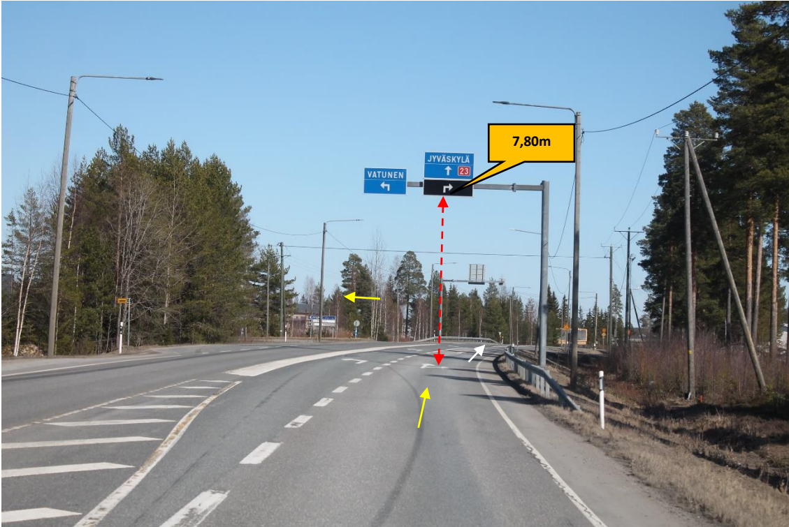
Pos 23/Pic 75. Turning from road 23 toward Vatusentie. https://goo.gl/maps/fCDyKbaw3zcksk2X7 Towers and other loads height over 4,5m need to use detour. Yellow arrow points driving direction for towers. White arrow points driving direction for blades.
